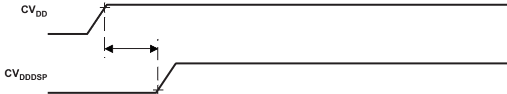
Figure 6-4. DSP Host-Boot Mode Core Supply Timings
