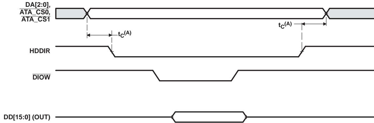
Figure 6-38. ATA/CF HDDIR Taskfile Write/Single PIO Write Timing
